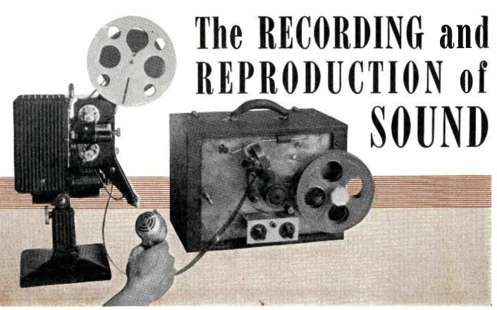
Fig. 1. A 16 mm. Filmgraph recorder in operation with home movie projector.
