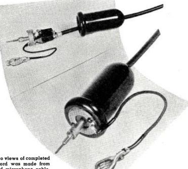
Fig. 1. Two views of completed probe. Cord was made from a shielded microphone cable.
