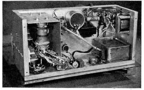
Fig. 4. Under chassis view of r.f. section shows relative placement of components.
