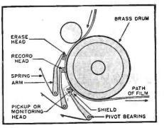
Fig. 9. Triple head assembly for recording and reproducing (magnetically) on film.
