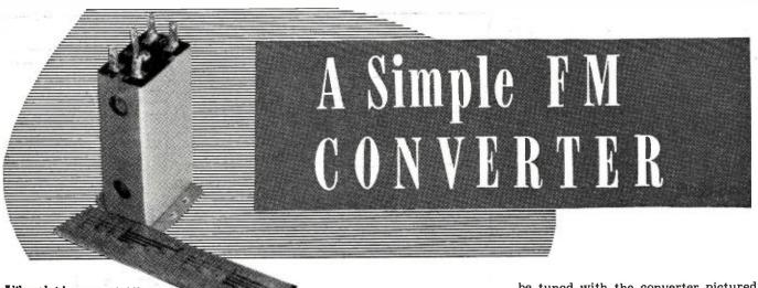
Although trimmers are preset, holes are provided in the case for later adjustments if found necessary.
