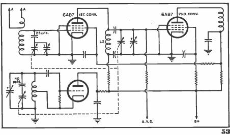
Fig. 7. Schematic diagram of the front end of the JFM-90 tuner after conversion. The oscillator tube is a 7A4. See Fig. 9 for complete coil specifications.
