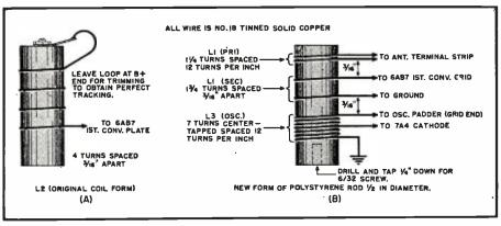
Fig. 9. Mechanical details of coil assembly for the General Electric JFM-90 tuner.
