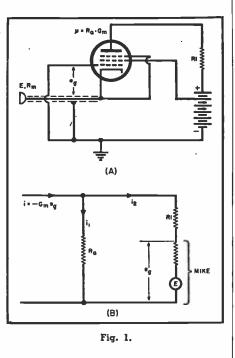
According to the formula, most pentodes, under recommended operating conditions, will be found to have an input impedance of around 1000 ohms in this circuit.
