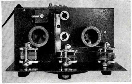
type. In these days of parts shortages this often entails considerable searching to locate the desired components. By the use of a regenerative second detector, however, it is possible to realize considerable gain. The use of a high frequency i.f. system insures adequate freedom from images.
