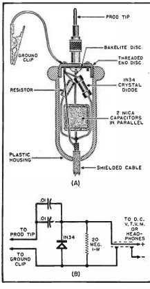
SYLVANIA 1N34 germanium crystal diode is the heart of the multi-purpose a.f.-r.f. probe shown in Fig. 1. This device will be useful to experimenters, amateurs, and servicemen. A crystal probe has the advantages that it can be made much more compact than the tube type probe, it requires no power supply of any kind, and it is free from the contact potential effects common to diode tubes. The 1N34 crystal diode may be used entirely safely whenever the inverse peak voltage does not exceed 50 volts.
