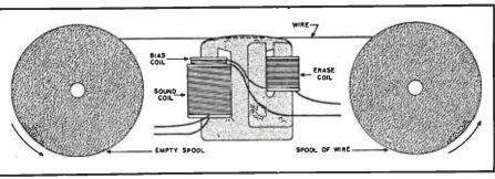
Fig. 11. Combined record-playback head assembly for wire.
