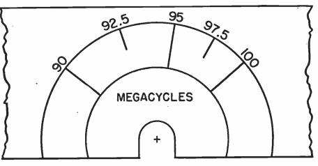
Full scale drawing of recalibrated dial scale for GE tuner.
