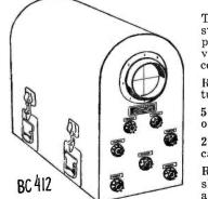
5" RECEIVER INDICATOR OSCILLOSCOPE WITH 31 TUBES
